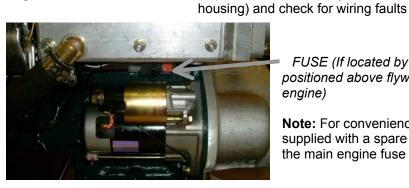
FUSE (If located by starter motor, usually it is positioned above flywheel housing at rear of engine)
