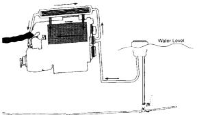
5. If water is required for stern tube lubrication then this should be taken from a 'T' piece in the pipe going from the heat exchanger outlet to the water injection bend.
