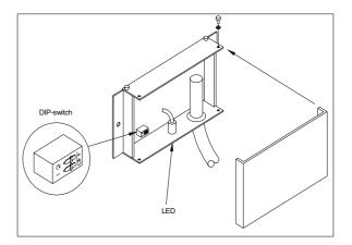
Cover removal for resetting of DIP switches
